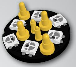
In any case, you should always use a connector casing to protect the integrity of both the pins (the blade will actually rest on the casing and not the pin's body) and the pixels.
