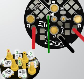
Blade on D1 (# of pixels in your blade : 0 to #) Connector on D1 (3 pixels : 0 to 2) mimicking first 3 pixels of Blad
