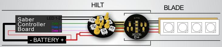
This diagram is a basic representation of the wiring you will have to do in order to use your connector in your saber. Detailes witing diagrams are located at the end of this manual. The summarised table in the next chapter helps you find the proper diagram for your actual saber install.
